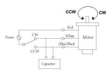
Rotation direction switch (1 phase motor):
